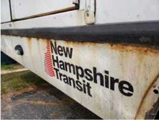
SCS: Corrosion on lower panel/wheel well
