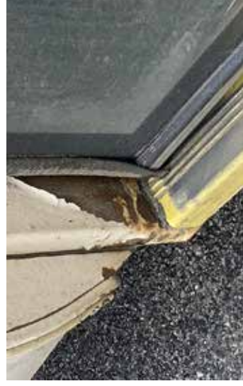
VNA@HCS: Corrosion affecting passenger door
