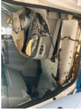
TCCAP: Damage to driver's seat
